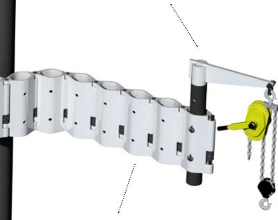
The JibFlex can be extended to reach out 7 m from the anchoring point. In this working radius, it can carry up to 150 kg. In a 3 m working radius, it can carry up to 500 kg. Please note that the working load limit (WLL) is defined as the payload plus the weight of the hoist mechanism.
